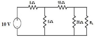
(b) Using Norton's theorem, find the current through the load resistor R in the following circuit. Draw the respective Norton's equivalent circuit. [(CO2)(Apply/IOCQ)]
