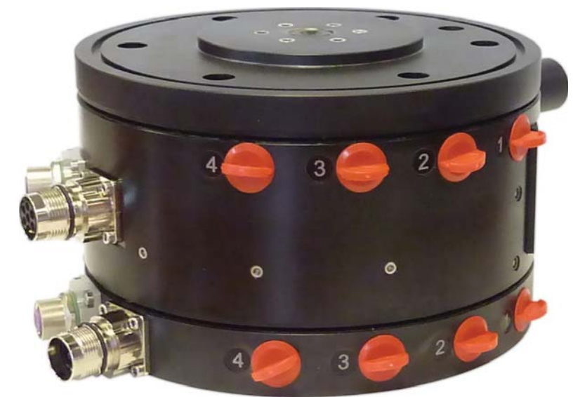
An 8-channel pneumatic Moog Rotokombi consisting of a Rotopack rotary union and Rotoflux slip ring used between a robot arm and tool for rotations of more than 360 deg. and precision clamping. Images courtesy of Moog GAT GmbH
