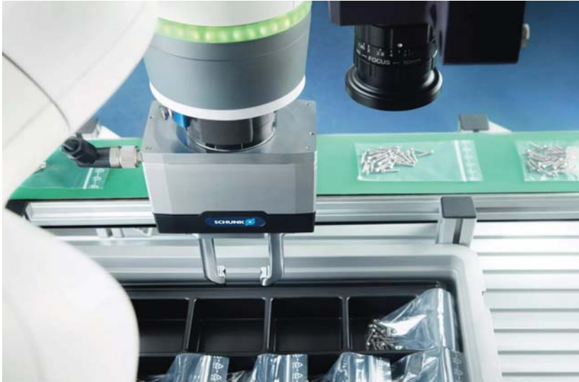
The winner of the 2024 Hermes Award, Schunk's 2D Grasping Kit is an intelligent solution for handling different non-position-oriented objects on a surface. Schunk
