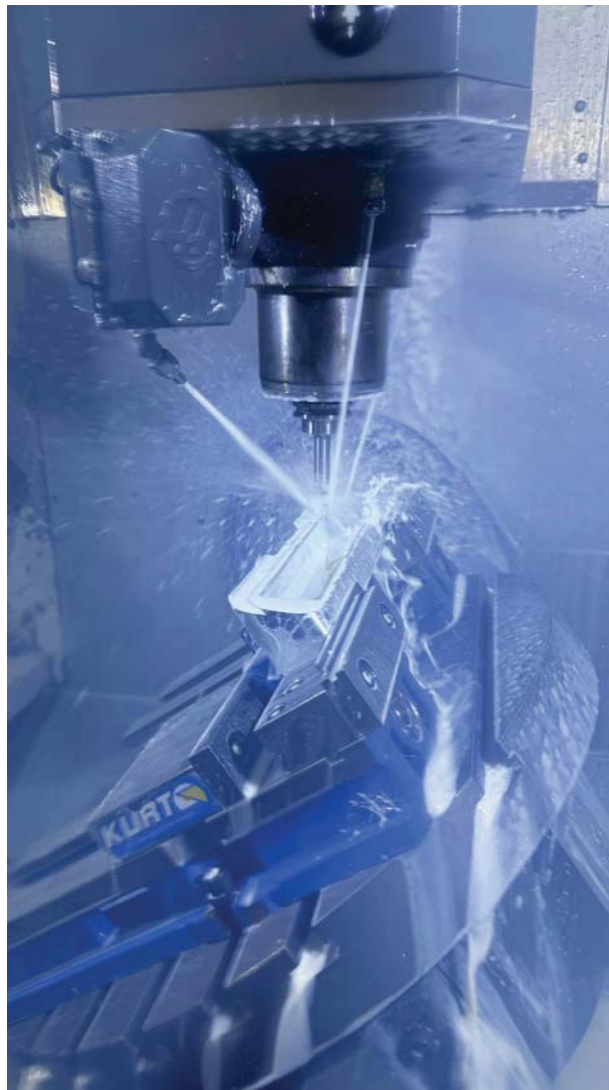
Kibbetech machines more than third brake lights using its 5-axis HAAS UMC-1000 CNC machine after the successful installation on a prerunner build helped create the demand. Kevin Strom
