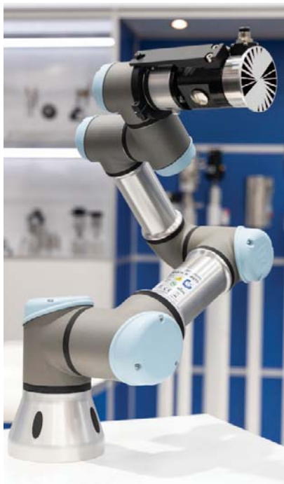
A Universal Robots UR3e with the Rotokombi solution on the end of the robot arm.
