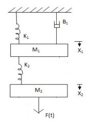
(b) Hence find the transfer function  $X_1(s)/F(s)$  where F(t) is the applied force and  $X_1(t)$  and  $X_2(t)$  are the displacement of mass  $M_1$  and  $M_2$  respectively.
