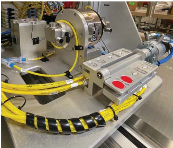
The aluminum housing of the industrial electronic component is mounted on a machine prior to assembly. A round opening is pointing up ready for the insertion of a plastic cover.
