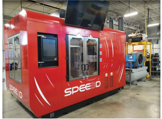
The WarpSPEE3D printer. Courtesy Bradley Deuser, Missouri S&T
