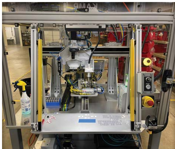
The operator's view of the adhesive machine showing the X, Y and Z axes.
