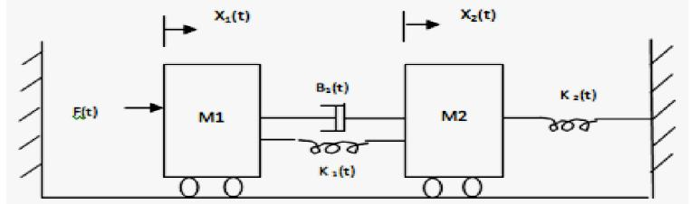
Draw the free body diagram of the masses in the given system and represent the system in terms of differential equations considering  $fc_1$  and  $fc_2$  as frictional coefficients for the mass M1 and M2, where F(t) is the applied force and X<sub>2</sub>(t) is the displacement of mass M<sub>2</sub>. [(CO1)(Analyse/IOCQ)]
