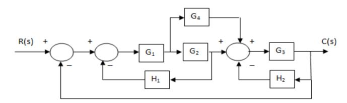
Find out the overall transfer function of the system for the given block diagram using block reduction technique. [(CO2)(Analyze/IOCQ)]
