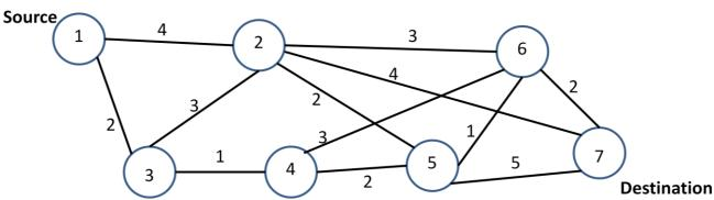
In the above AdHoc wireless communication network using Wireless Routing Protocol (WRP), with Node 1 as source and Node 7 as destination, find the table of routing entry at each node for the destination Node 7 showing the (i) Node id, (ii) Successor node id, (iii) Predecessor node, and (iv) and the Cost involved as each table row entry.
