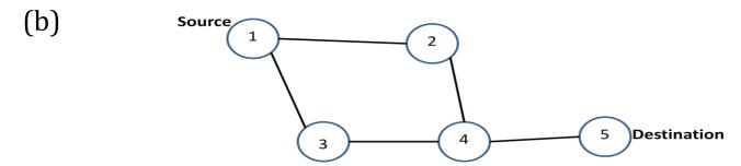
Using the above AdHoc wireless communication network explain the route establishment between Source Node 1 and Destination Node 5 with Dynamic Source Routing (DSR) protocol using RREQ (route requests) packet and RREP (route reply) packet paths.
