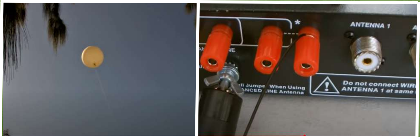
Pic 1 shows the balloon at a height of approximately 100 feet. This technique is used for end-fed long wire antennas. It is a single wire connection. The antenna wire is connected to the marked port of the HF transceiver set. Pic 2 shows the long wire antenna, connected to the designated port.
