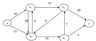
Apply FORD-FULKERSON algorithm on the above flow network to find the maximum flow in the network. s & t denote the source & destination respectively and the capacity associated with every edge is given along with the edge. What is the running time of this algorithm in the worst case considering arbitrary (positive) capacity values? [(CO3)(Apply/IOCQ)]
