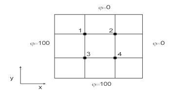
From the above figure, where  $\phi$  is governed by  $\text{div}(\rho u \phi) = \text{div}(\Gamma \text{grad} \phi) + a - b \phi$ , where  $\rho$ =1,  $\Gamma$ =1, a=10 and b=2.  $\Delta x$ = $\Delta y$ =1. The flow in the x-direction=u=1 and the flow in the y-direction=v=4. Using upwind scheme find out values for  $\phi_1$ ,  $\phi_2$ ,  $\phi_3$ , and  $\phi_4$ . [(CO3)(Apply/IOCQ)]
