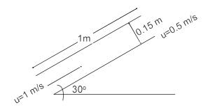
A liquid of density 1000 kg/m³ and viscosity 0.001 Pa.s is flowing over the inclined plane as shown in the above figure. Using artificial compressibility method, develop a solution matrix for evaluating pressure and velocity at three intermediate nodes. Assume the flow is in streamlined condition. Given: Sound velocity=1520 m/s. [(CO4)(Apply/IOCQ)]
