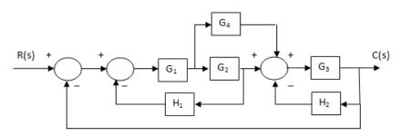
Find out the overall transfer function of the system for the given block diagram using block reduction technique. [(CO2)(Analyze/IOCQ)]
