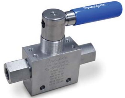
The trunnion-style ball features an innovative direct-load design to enable leak-tight performance and a bottom-loaded stem design to eliminate stem blowout.
