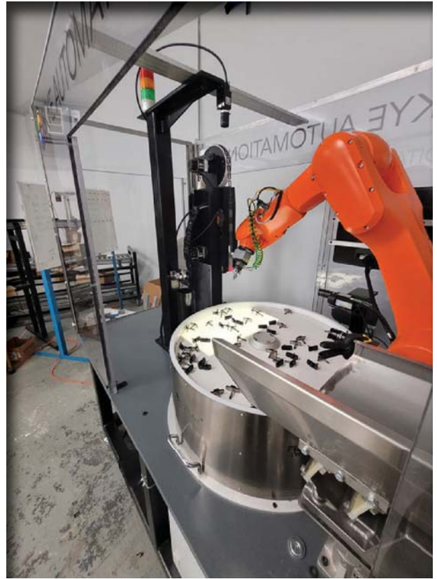
The FlexiBowl is a flexible bulk feeder supported by a vision system and calibrated to an industrial robot. It is suitable in applications where there are frequent changeovers. Credit: Skye Automation
