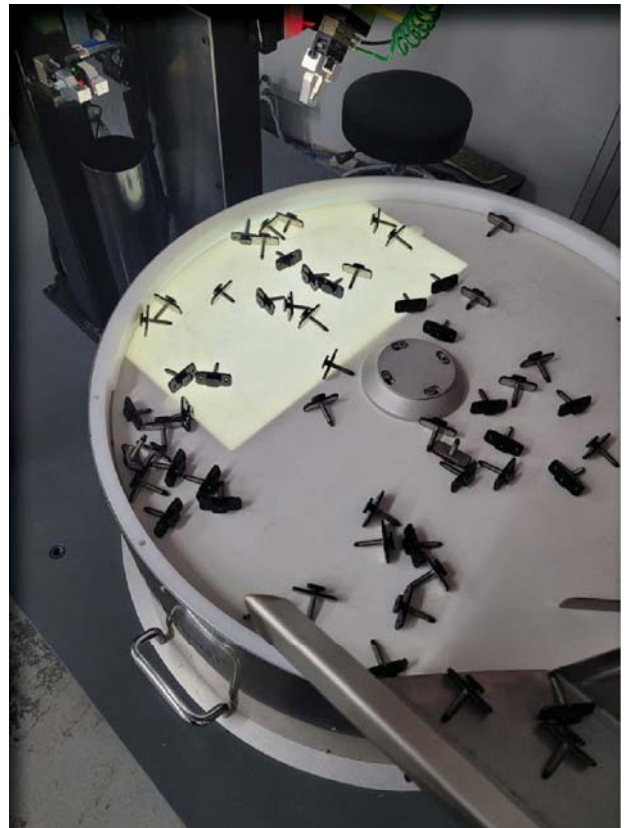
The FlexiBowl's achieved feed rate is between 20 and 50 parts per minute and has a high payload, with parts total weight exceeding 7 kg. Credit: Skye Automation
