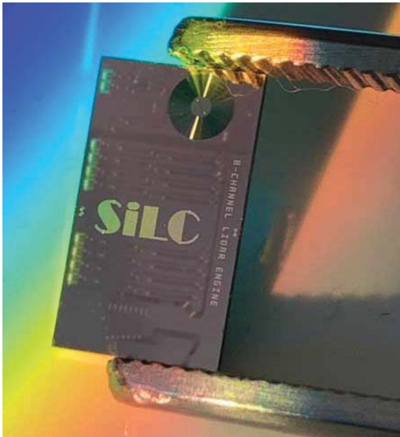
The Eyeonic Vision Sensor is a silicon photonic chip the size of a thumbnail.
