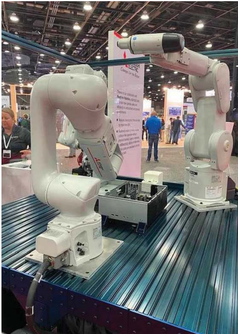
At the Mitsubishi booth, two robots (RV-7FRL and RV-8CRL) simulated their ability to move to various focal points on a workpiece, while the ASSISTA collaborative robot worked around them to inspect various points of interest. Credit: Mitsubishi
