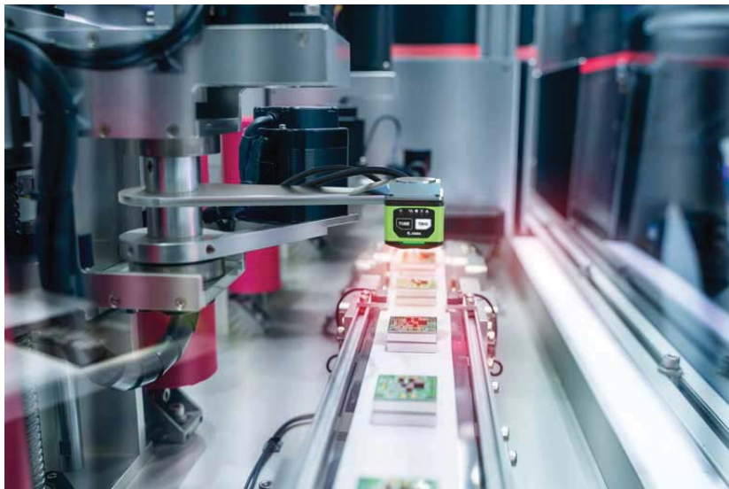
Zebra’s VS40 shown in a vision application. Quality inspections and track-and-trace cameras can be tailored to business needs. Options include range, illumination, connectivity and power. Credit: Zebra Technologies
