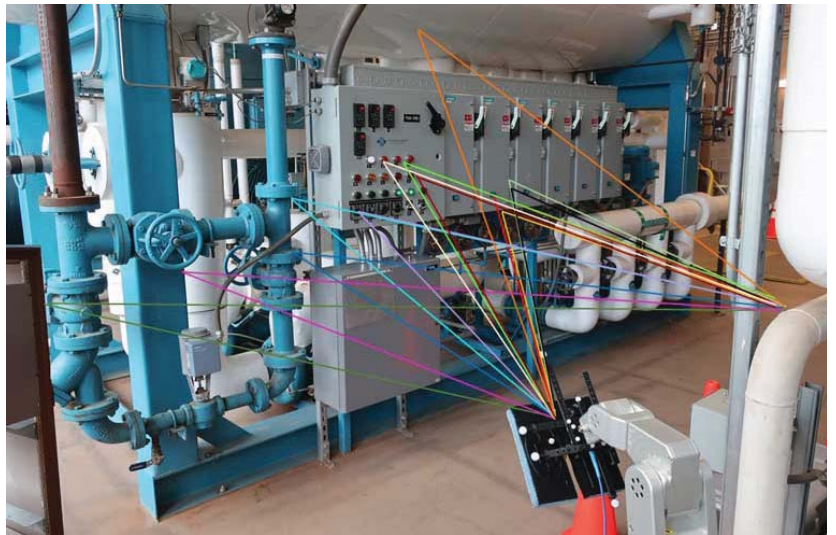
Wireless transmissions can take many different routes to the intended receiver. The colored lines are reconstructions of measured paths of millimeter-wave signals between a transmitter (not visible) and receiver (lower middle) in a NIST industrial control room. These paths are all secondary, meaning they are reflected or diffracted signals. Credit: NIST
