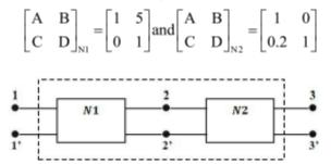
Find the overall parameters of the combined network. [(CO2), Understand/IOCQ]
