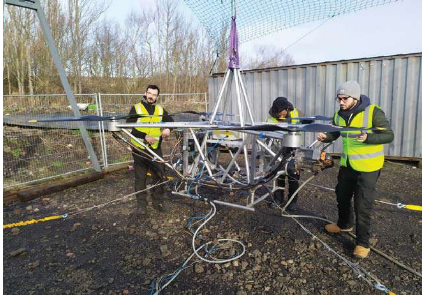
The Flowcopter drone can fly for more than six hours, up to 900 km. Hydraulic motors are sealed, and are proven workhorses in offshore environments. Images: Flowcopter Inc.
