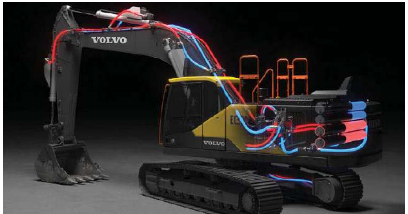
Volvo’s ground-breaking electrohydraulic system achieved radical improvements in energy efficiency. Image: Volvo Construction Equipment
