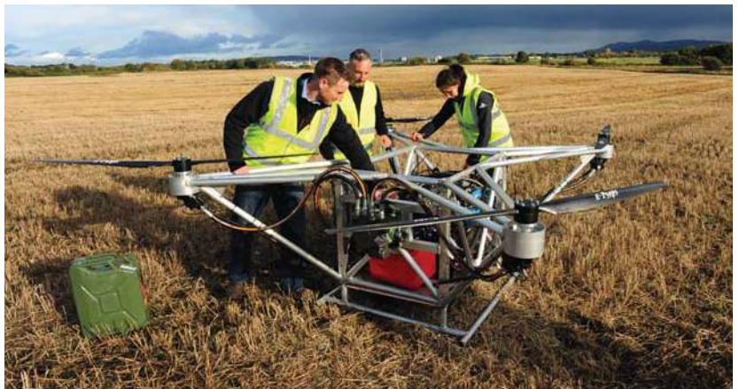
The Flowcopter drone can fly for more than six hours, up to 900 km. Hydraulic motors are sealed, and are proven workhorses in offshore environments. Images: Flowcopter Inc.
