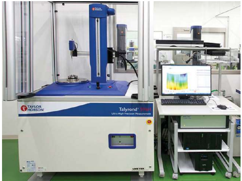
This CNC roundness measurement machine measures workpiece diameters to an accuracy of 0.015 +0.0003 μm per millimeter. Image: AOMI Precision
