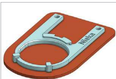
FFF parts are usually printed on a raft (in red) which helps maintain dimensional accuracy during sintering.
