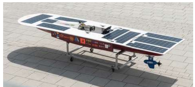
Students at an engineering school in Poland designed a solar-powered boat that included lubrication-free and seawater-resistant bearings from igus. igus
