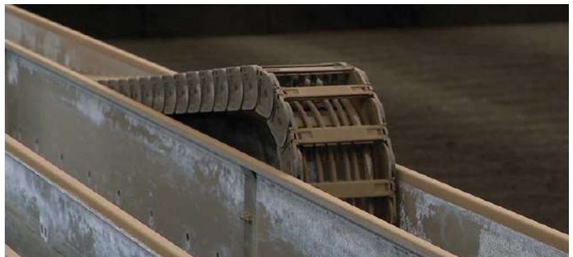
The HUBER Sludge Turner SOLSTICE units work in greenhouses, and the turner travels on rails and repeatedly rearranges the sludge on the ground. During the movement, the sludge is dried by solar energy. The system takes a solid mixture that is 78% moisture and water and 22% dry solids and converts it to 75% dry solids. igus
