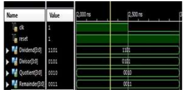
Fig.11 Division of 13 by 5 using restoring division
