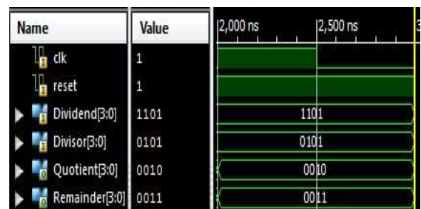
Fig.15 Division of 13 by 5 using non-restoring division
