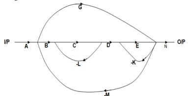
(b) Find the overall transfer function of a system having the following block diagram using block reduction technique.
