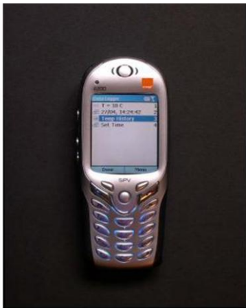
Figure 9 – The Temperature Logger user interface on a Smartphone.
