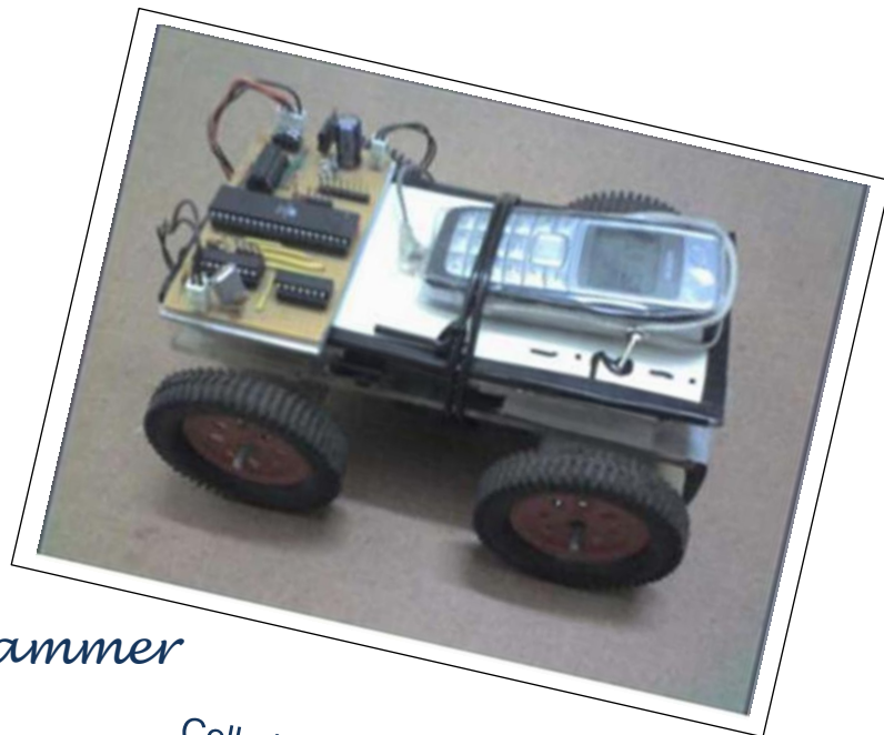
Cell phone operated Land Rover
