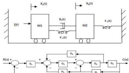
Find the overall transfer function of the system for the given block diagram using block reduction technique. 6+6=12
