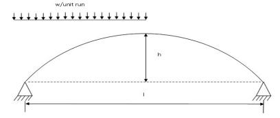
(b) A two hinged parabolic arch of span 18m and rise 3.6m carries two concentrated loads of 25kN each at the crown and at the left quarter span section. Find the horizontal thrust at each support and the bending moments at the loaded sections. Assume secant variation of moment of inertia of the arch section.
