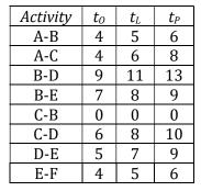
(b) If the schedule completion time is 30 days, determine the slack time for each event and identify the critical path. Enter the values in a tabular form.
