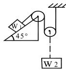
Please refer to the figure given below. The system is released from rest (b) with the spring initially stretched 75 mm. Calculate the velocity v of the weight after it has further dropped by 12 mm from stretched position. The spring has a stiffness of 1050 N/m. Neglect the mass of the small pulley.
