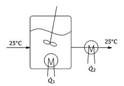
The feed concentration,  $C_{Af}$ , is 4 mol/L and feed flowrate,  $Q_{f}$ , is 250 L/min. The reaction-rate constants have been determined experimentally
