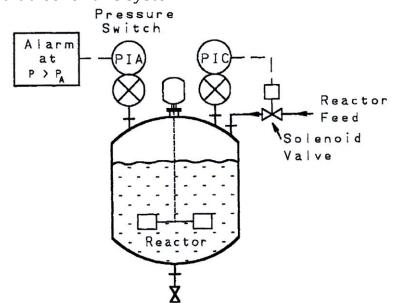
This reactor contains a high-pressure alarm to alert the operator in the event of dangerous reactor pressures. It consists of a pressure switch within the reactor connected to an alarm light indicator. For additional safety an automatic high-pressure reactor shutdown system is installed. This system is activated at a pressure somewhat higher than the alarm system and consists of a pressure switch connected to a solenoid
